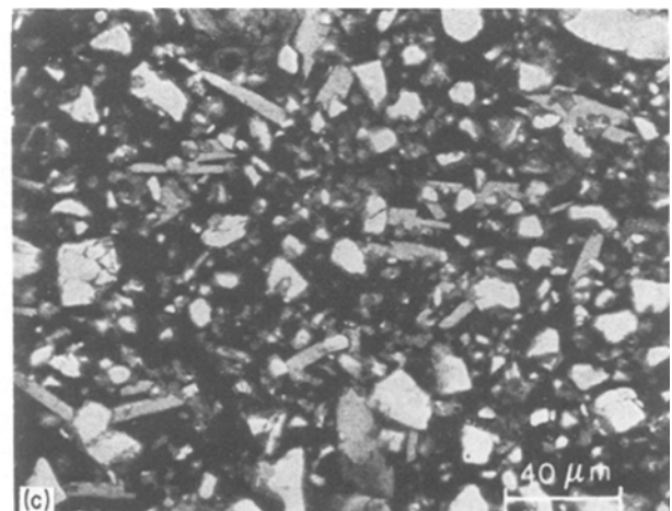
Figure 3 Micrographs of 3 day specimen, using backscattered electrons, of polished alite. White— \text{Ca(OH)}_2 ; light grey—alite; medium grey— \text{Ca(OH)}_2 ; darker grey—C-S-H; darkest grey—epoxy.
